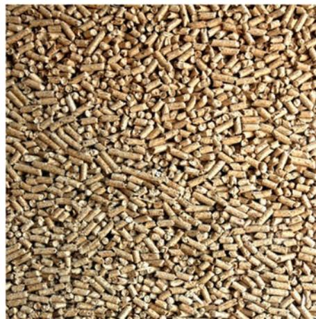
**Fig. 3** Wood pellets. Photo courtesy of Böhlinger, Wikimedia Commons.
